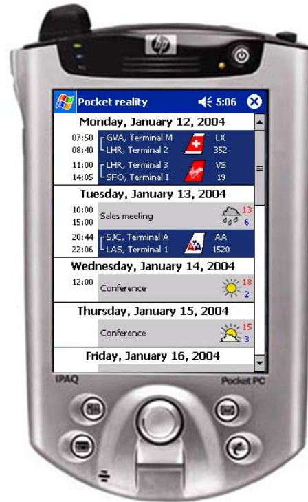
Figure 1: The different activities of the User Task Model are displayed chronologically from top to bottom. The current one is highlighted and past ones are grayed out.
